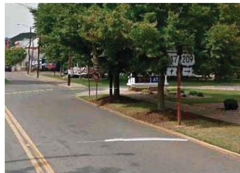
If a detour requires Route 147 to close down and all traffic to turn right, the municipality should make sure the route shield directional sign for Route 147 at this intersection is covered. (Image courtesy of Google Earth.)
