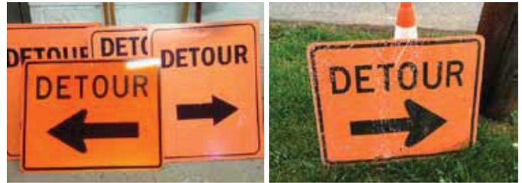
Which detour sign is properly maintained and meets retroreflectivity requirements? If you picked the front sign in the photo at left, you are correct.
